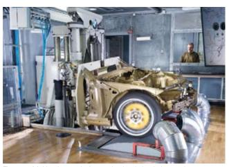
Figure 2: Multi-axis test rig for service load simulation testing (picture: © IABG)
