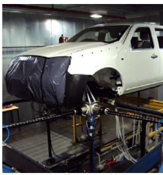
Figure 2: Multi-axis FlexMAST test rig (picture: © Ford)
