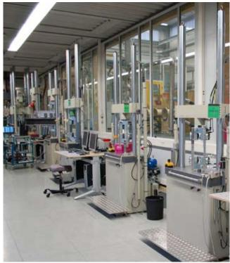
Figure 1: Modernized servo-hydraulic testing machines
