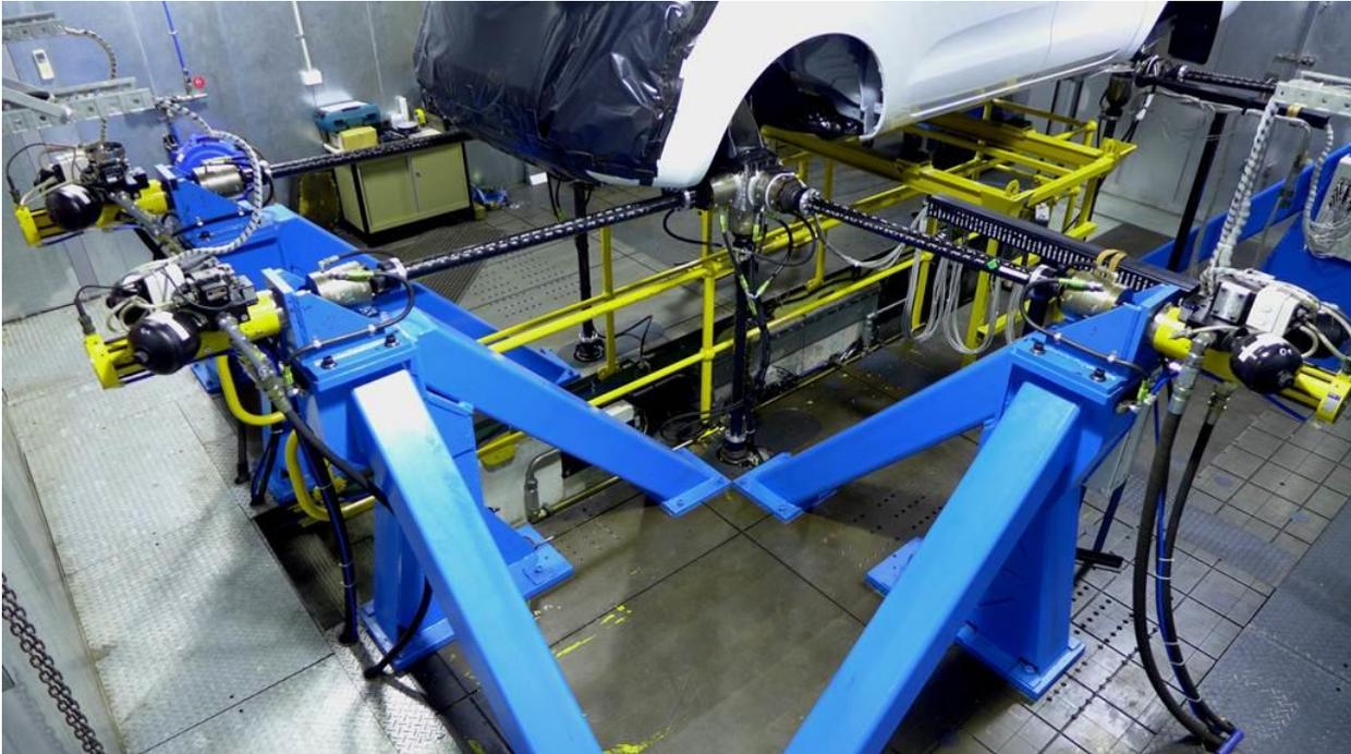
QanTiM simulation testing enables you to bring greater realism, accuracy and repeatability to mechanical testing. Laboratory testing helps shorten your product development cycle for structures or components. QanTiM simulation enables you to reproduce the actual real-time loading conditions for a vehicle or structure in a test laboratory. Real-Time Simulation Testing offers the only method of reliably conducting interactive multi-axis tests.
