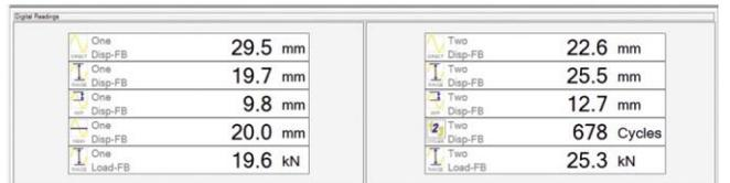
**Virtual Transducers** - allows you to enter a mathematical equation for computed (virtual) channels, which may be applied as monitor or control loop feedbacks. Features such as digital display, strip chart, acquisition, limits etc. are also supported with virtual channels. Runs at full 4096 Hz system rate.
